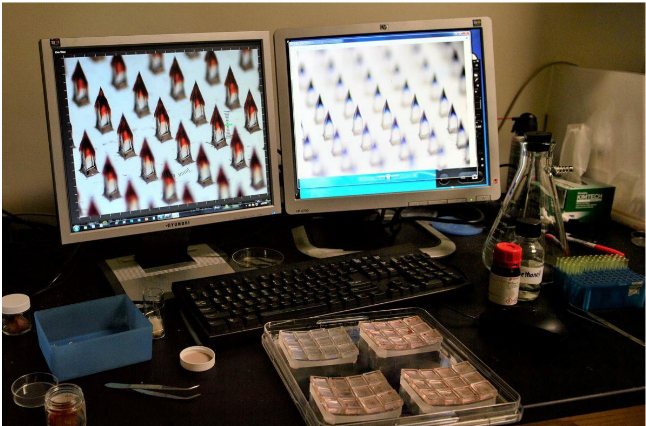
These screens show a magnified view of the PittCoVacc's microneedle array. Photo courtesy the University of Pittsburgh School of Medicine
